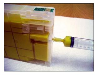
bottom of the cartridge and so it is not necessary to remove the air from the ink exit port.
