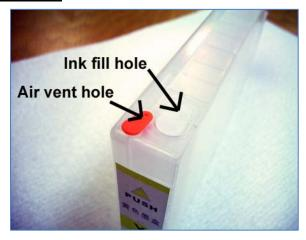
The only time you should have this bung in place when the cartridge is installed in the printer is if you intend to not use your machine for an extended period – inserting the bung will stop any ink evaporation during extended periods of non-use.
