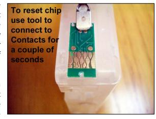
cartridge. If you don't refill the cartridge to full when resetting the cartridge chip to full, then the ink level on the machine display will be out of sync with the actual ink level in the cartridge, and the cartridge could run dry before the printer display shows it as low or empty.
