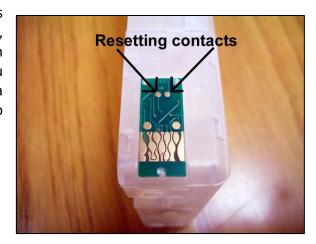
After resetting the chip and re-installing the cartridge, the printer display should show the ink level at 100% for the reset cartridge. If not, remove the cartridge and try resetting the chip again. Chips can be reset to full using this method at any time, so even a cartridge that is still showing 75% full, for example, can be refilled and reset prior to a long print run if required.
