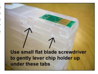
To install the new chip, simply line up the chip holder assembly over the recess in the cartridge and push down on the side of the plastic to snap the new assembly into place. Try to avoid touching the gold contacts on the chip during this operation. After a chip has been changed, it is wise to purchase a new spare chip from your supplier.
