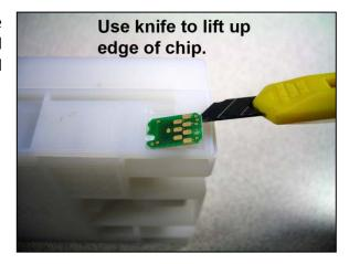
Take the refillable cartridge that corresponds to the color of the original chip you have just removed, and remove the bridge chip from the cartridge. Removing the bridge chip is very simple – simply use a small screw driver to lever up the plastic at the end of the bridge chip as in this picture. Once you have levered up the end of the plastic, the bridge chip can be completely removed from the cartridge.
