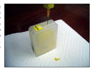
Refill the syringe and continue injecting ink into the cartridge until the cartridge is full. It will take nearly three complete syringes full of ink to fill the cartridge. Use paper towel to wipe any ink from the surface of the cartridge, and return any ink in the syringe back to the correct color bottle.
