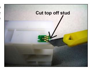
Once you have trimmed off the top of the plastic stud, use the knife to lift up the edge of the chip. The chip can now be pulled off the original cartridge. Try to avoid touching the gold contacts on the chip when handling it.
